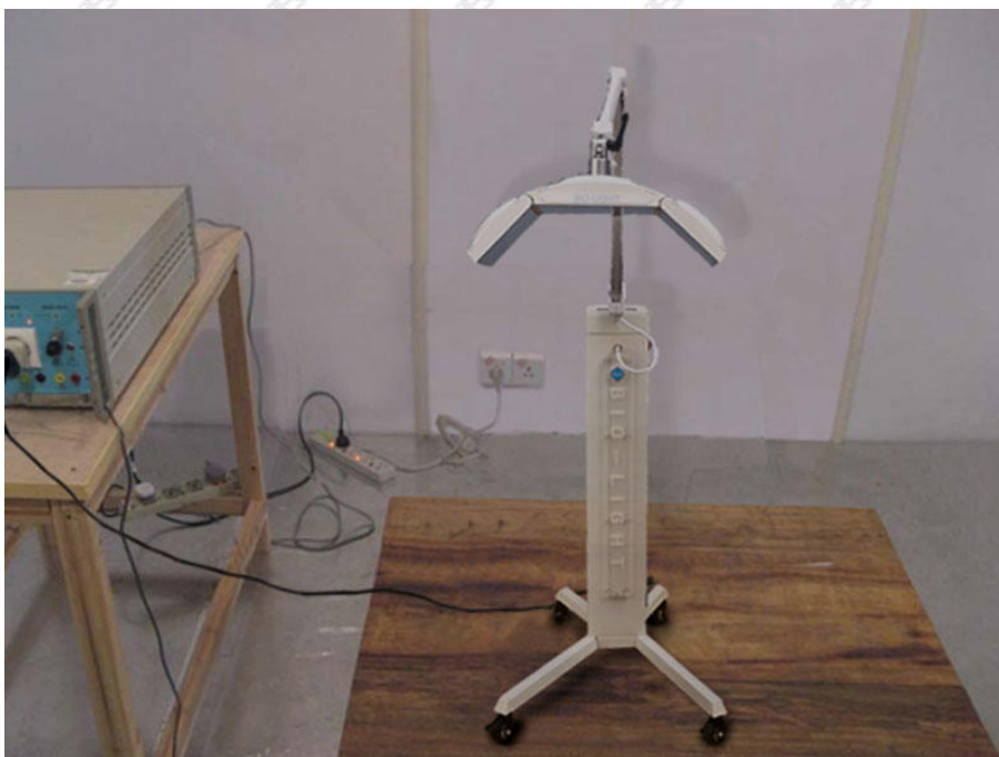
EN 61000-3-2 POWER HARMONICS & EN 61000-3-3 VOLTAGE FLUCTUATION/Flicker TEST SETUP
